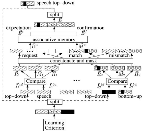
Figure 6: Generation of the teaching signal for the online-speech learning. At the bottom the expectation for one feature channel (e.g. position) is generated from a specific utterance (e.g. 'learn where this object is'). This top-down expectation is propagated through the loop in the standard way (see Figure 5) and generates the teaching signal for the speech shown at the top.
